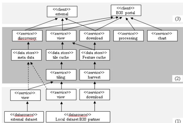
Figure 2 – EGS architecture with (1) data/service provider, (2) central EGS implemented in the cloud and (3) service consumer.
